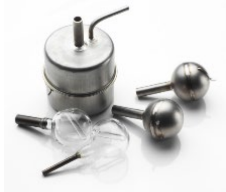
Figure 2: Typical ARC cells
